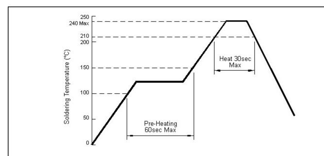
Fig 1 – Temperature profile of Reflow Soldering at 250°C Max.
