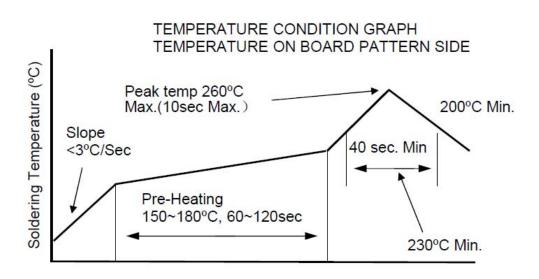
Fig 1 – Temperature profile of Reflow Soldering at 260°C Max.
