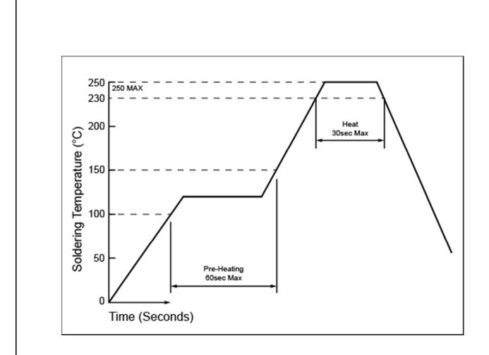
Fig. 1. Recommended Reflow Temp. Profile
