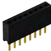
BD080 1.27mm pitch 03 - 40 contacts 4.30mm profile
