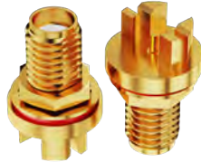
RFPC-SMA23-FN IP68/69K Edge Mount DC to 6GHz Brass, Gold Plated
